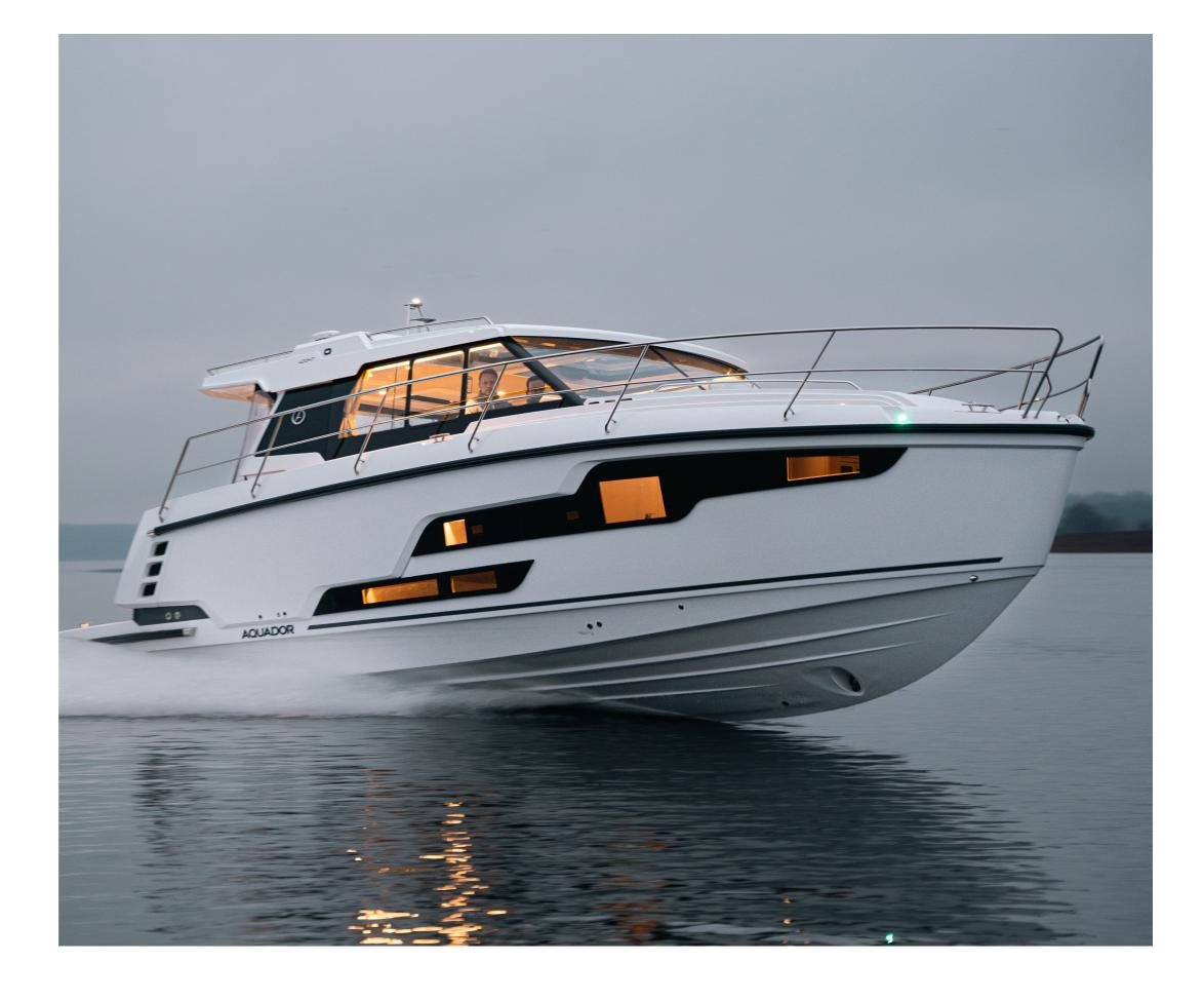
Aquador's Aquadynamic hull allows planing at lower speeds and much less power is required to reach cruising speed, leading to greater fuel economy especially on longer passages. More stability is achieved in turning and the sharp attack angle at the bow means a softer ride.
